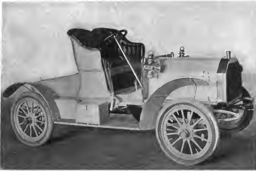
GROUT GASOLINE RUNABOUT, FITTED WITH TURTLE BACK.
